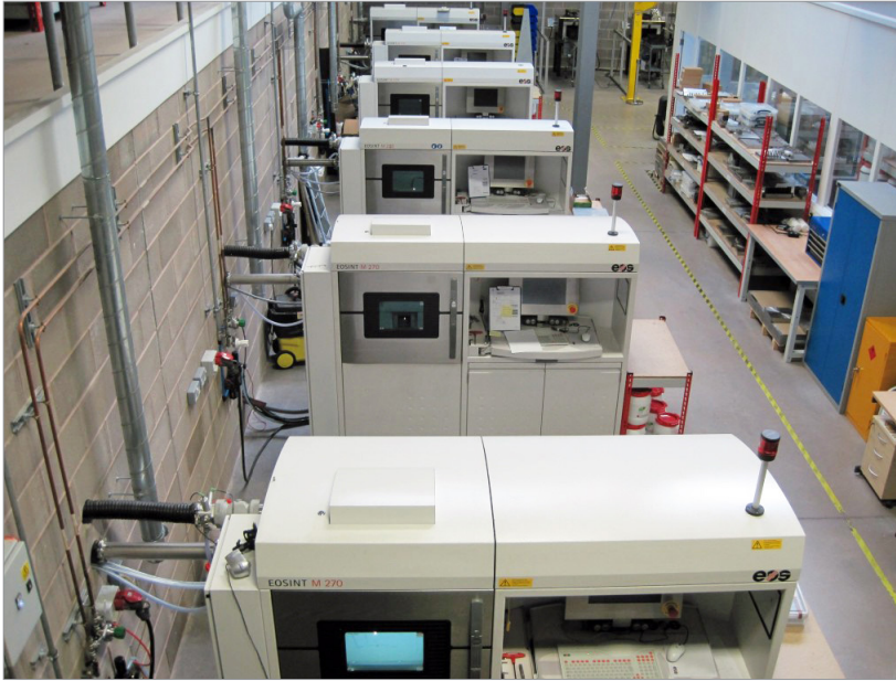
Fig. 2 Materials Solutions currently operates eight EOS machines, with a further three due to arrive this year
